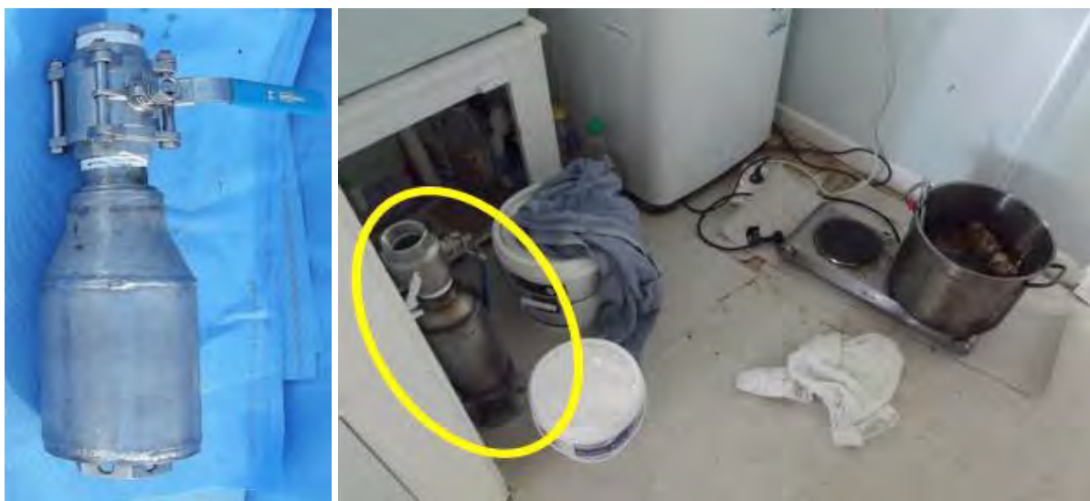
Figure 3: Parr Bombs – Pressure reaction vessels used to carry out the manufacture of methamphetamine in New Zealand.
