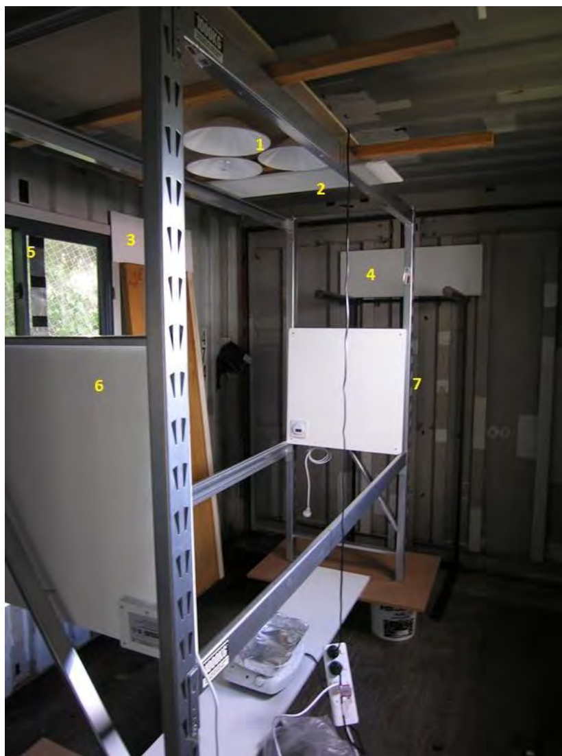
Photograph 17: Container smoking experiment – Three light shades including one with a working bulb (1), painted plasterboard (2,3), metal-painted (4), metal-bare (5), panel heaters (6,7).
